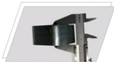
厚板亮面切割 BRIGHT SURFACE CUTTING OF THICK PLATE
