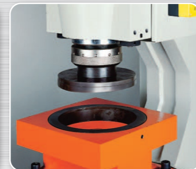
*Oversize punch attachment. Safety cover removed for showing.
